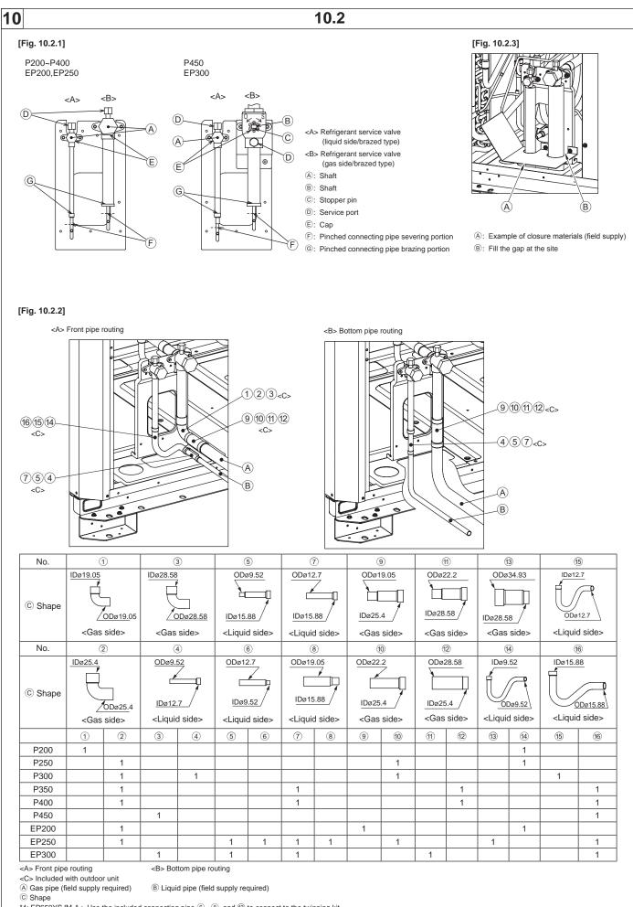
\*4: EP650YSJM-A : Use the included connecting pipe (6), (8), and (13) to connect to the twinning kit. \*5: EP700YSJM-A1 : Use the included connecting pipe (6) to connect to the twinning kit.
