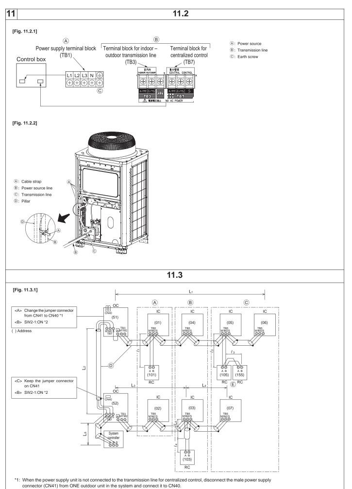
\*2: If a system controller is used, set SW2-1 on all of the outdoor units to ON.
